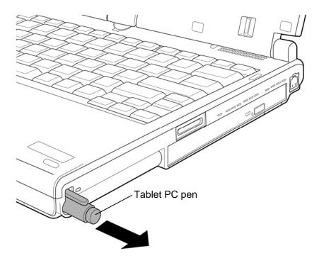
Figure 4-4 Removing the tablet PC pen
